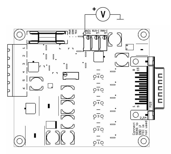
You can calculate the necessary voltage like this: 2.73V + (Temperature ℃ \* 0.01V) For example, you need to set the driver to 30℃: 2.73V + (30℃ \* 0.01V) = 3.03V
