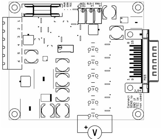
Each shunt has a resistance of 0.1 Ohm, so it's very easy to measure the current:
